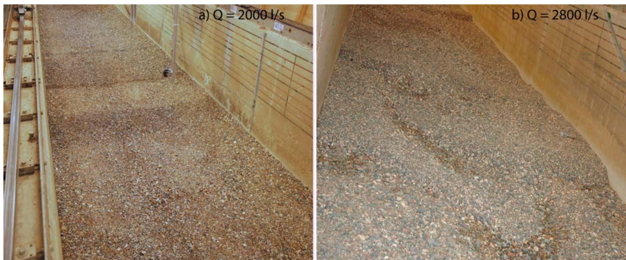
Figure 2. Photograph of bed surface at the end of the flow for the discharges of (a) 2000 L/s and (b) 2800 L/s. The direction of flow in both cases is from the top to the bottom of the photographs.
