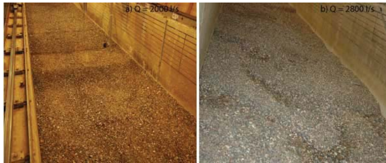
Figure 2. Photograph of bed surface at the end of the flow for the discharges of 2000 l/s (left), and 2800 l/s (right). The direction of flow in both cases is from the top to the bottom of the figures.
