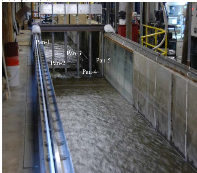
Figure 2. Weighing Pans located at the downstream end of the test channel. The experiment was conducted at the St. Anthony Falls Laboratory, National Center for Earth-surface Dynamics, University of Minnesota.
