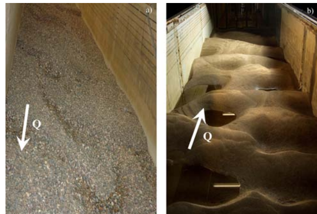
Figure 2. Bed forms formed in the main channel facility at the St. Anthony Falls Laboratory for (a) the gravel bed experiment at the discharge of 2800 L s -1 and (b) sand bed experiments at the discharge of 2500 L s -1 . The flow direction in Figure 2a is from top to bottom, and in Figure 2b it is from bottom to top.
