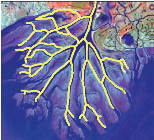
FIG. 1. Wax Lake delta. The skeleton network (yellow lines) is superimposed on the aerial view of the delta in 2005 by the National Center of Earth-surface Dynamics (NCED). Only links in the network that connect the delta apex to the shoreline outlets are considered in the connectivity analysis.
