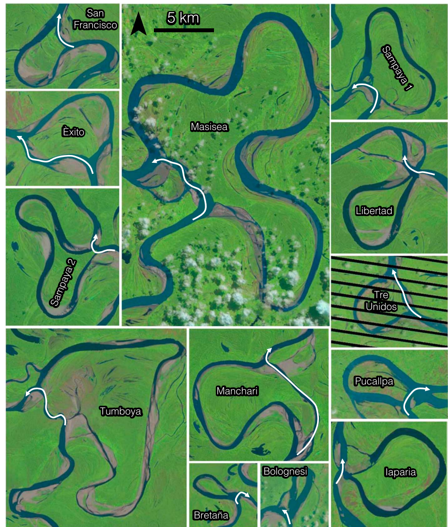
Figure 1. Cutoffs along the Ucayali River. Thirteen cutoff events along the Ucayali River during the period of 1985 to 2015 are shown midway through the cutoff process and at low flow. Chute channels and flow directions are denoted by white arrows. The north arrow and scale bar apply to all images. See Table 1 for more information on the cutoffs.
