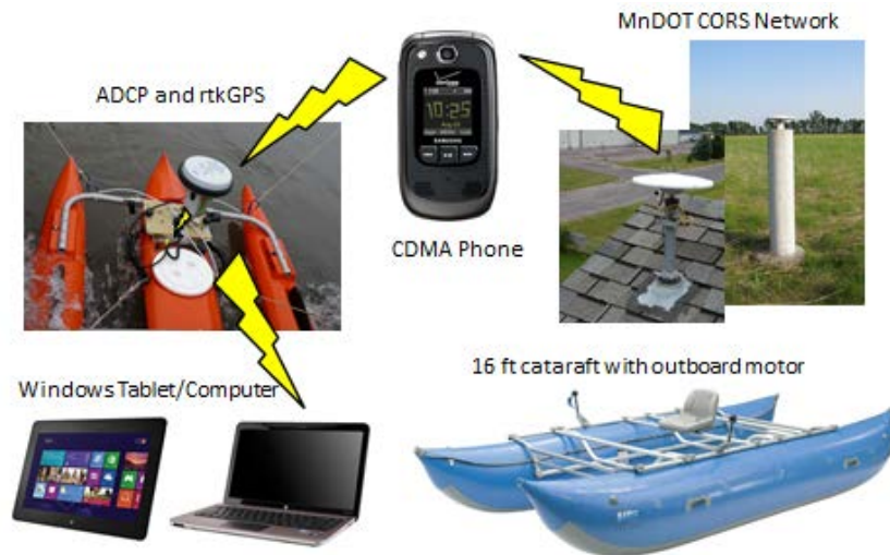
Figure 9. Top Panel: illustrates our system for rapid channel bathymetry mapping. Bottom Panel: show the 33 km reach of the mainstem Minnesota River that we were able to map in six days during summer 2013.
